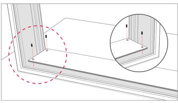
**2** Before installing the LEDs, screw the ACM panel to the bottom of the extrusion bar frame. (refer to Figure 1 on page 2).
