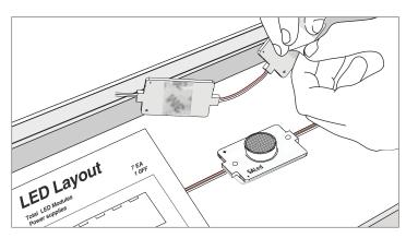
**3** Remove the tape from the back of the LEDs and stick them in **ACM panel** according to the provided layout (refer to Figure 1 on page 2).
