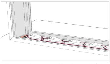
4 Ensure modules are connected in series or parallel (refer to Figure 2 on page 2). Avoid exceeding the maximum module count. WAGO connectors enable quick wiring of LEDs.
