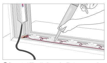
Secure the LEDs with silicone glue. Fix the power supply to the inside of the lightbox with screws, and wire both ends of the LED modules to the power supply (refer to page 2)
